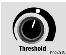
Located at the bottom left of the control panel, the **Threshold** control allows for adjustment of the background threshold level. This background “threshold” or “hum” aids in the location of targets. Small or large deep targets may not produce a distinct target signal but rather cause only a slight change in the threshold tone.
