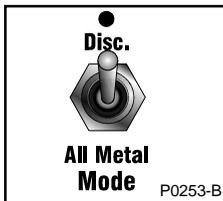
This switch is located in the centre of the control panel and is used to select **Disc.** (Discriminate) or **All Metals** mode. In **Disc.** mode, the **Disc** and **Notch** controls have become active and can be used in combination to ignore various unwanted metal objects.
