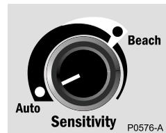
At the most anti-clockwise position this control “clicks” into the Auto position. In this setting the Sovereign Elite will automatically adjust the level of sensitivity to the most stable level under the prevailing conditions. Beginners should operate the unit in Auto, until they become more competent in its operation.
