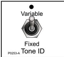
In the **Variable** position, the tone of audio signals received will change to help identify the object that has been detected. The lower an object's conductivity, the lower the pitch of the signal tone. For example, the pitch of a piece of aluminium foil will be lower than that of a gold coin.
